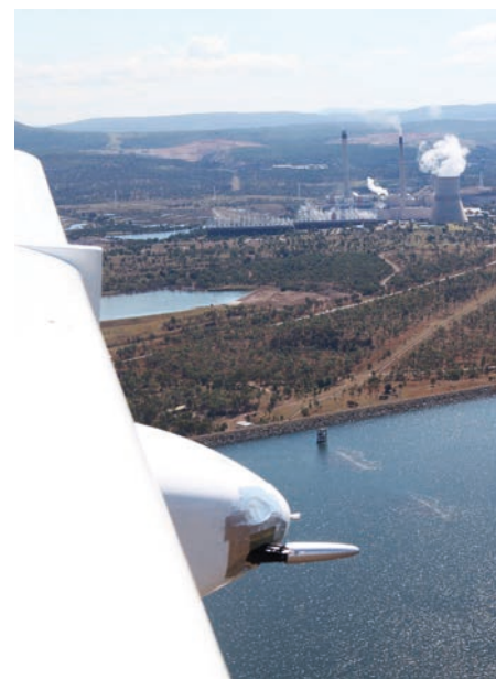
The particle inlet tube on an underwing pod, used to check ultrafine particle emissions from coal-fired power stations.
