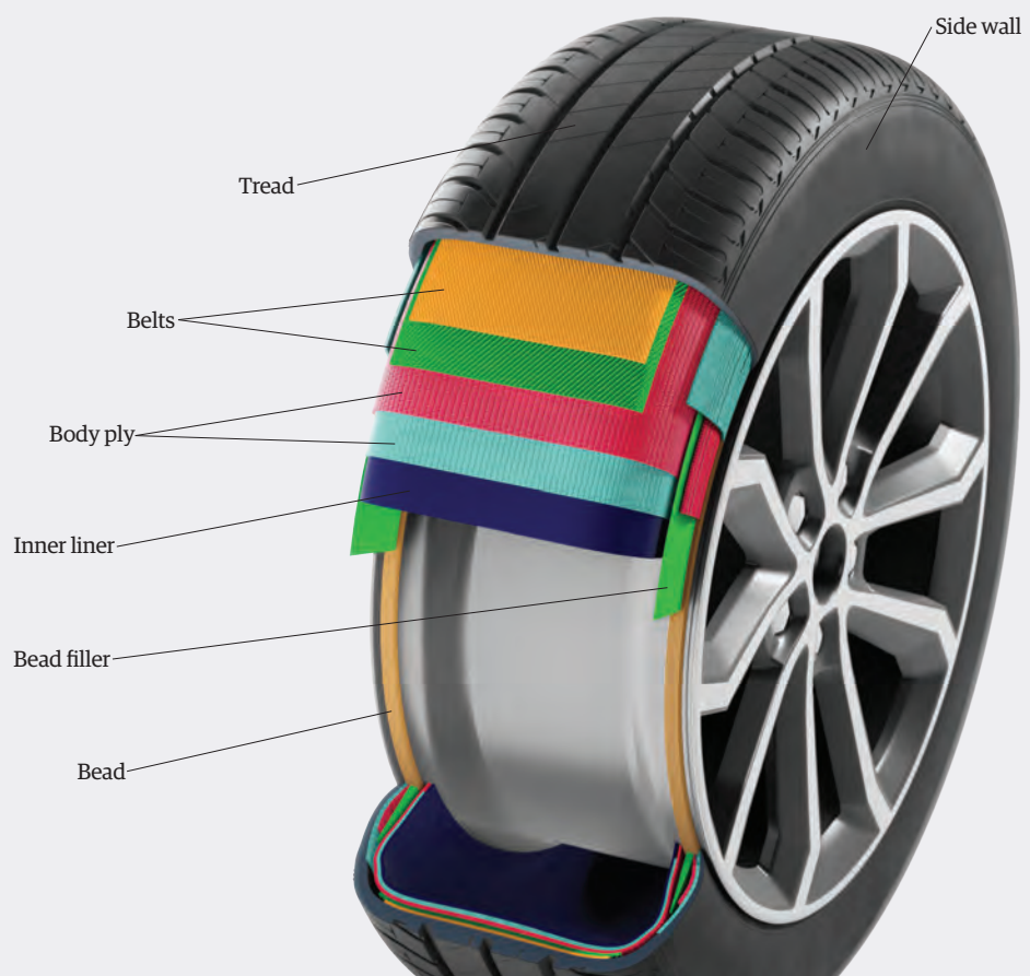
Tyre constituents by weight (above) and the internal structure of a typical tyre (below).
